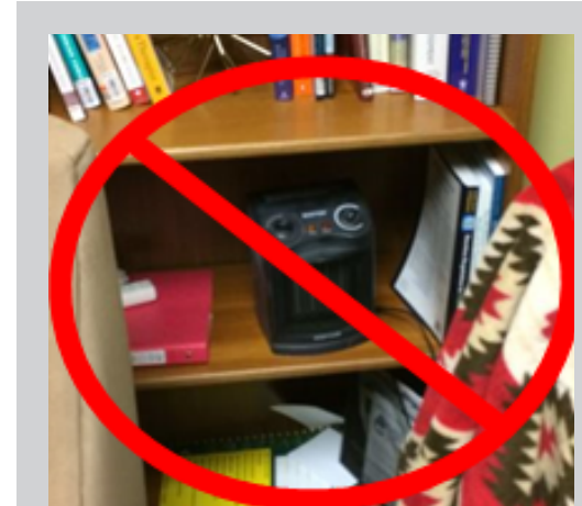
Keep flammables at least 3 feet from all sides of the space heater.
