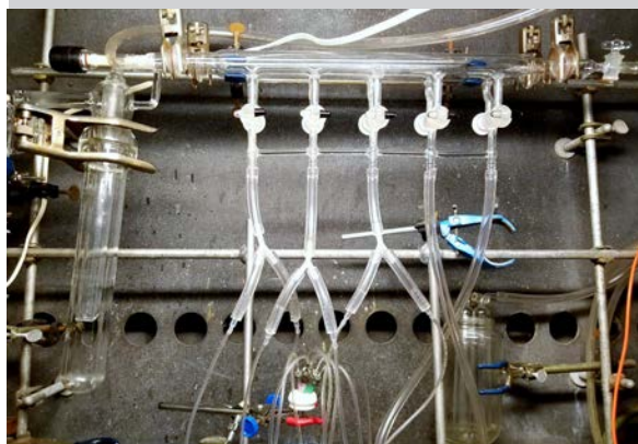
Example: Liquid trap. Always install to keep solids or liquids out of pump lines.
