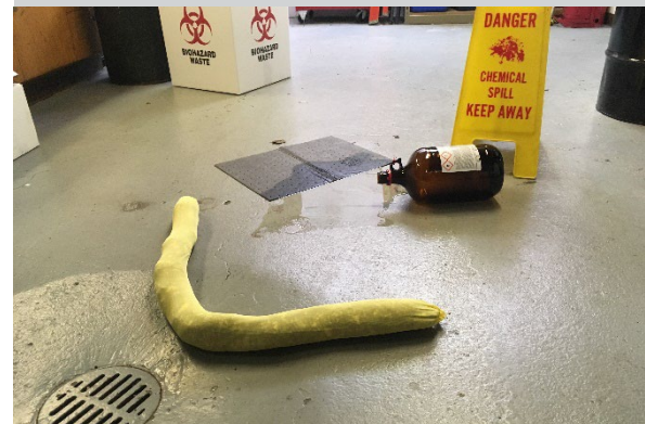
Prevent spills of potentially hazardous materials from entering sewer drains.
