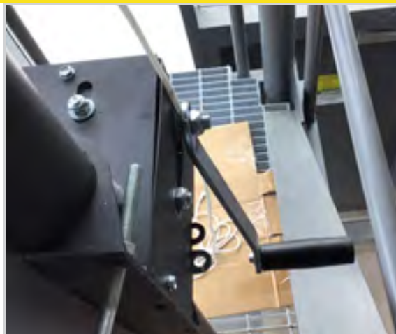
The tabs are not in alignment so the crank can be turned.
