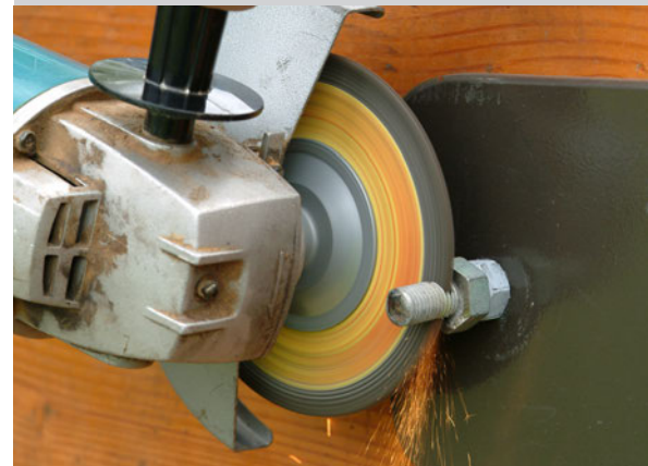
Ensure machine guards are secured in place before starting work!
