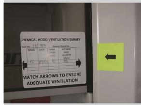
To ensure proper functionality align the arrow on the sash sticker to the arrow on the side of the hood during use.
