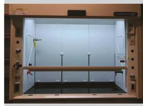
Keep fume hoods clear and minimize storage to provide adequate ventilation.
