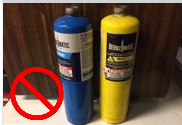
Do not store propane inside a flammable cabinet!
