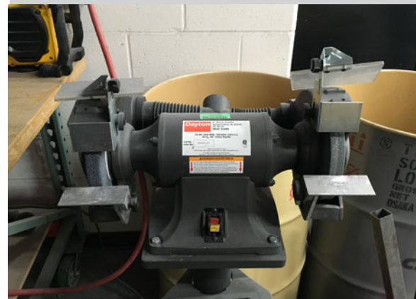
Keep guards in place!
