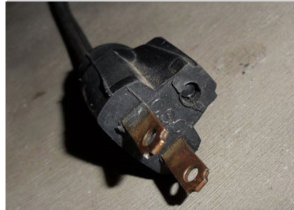
Do a pre-use inspection for damage!
