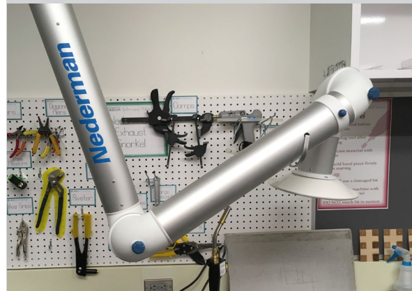
Utilize a fume hood or local exhaust to capture WAGs
