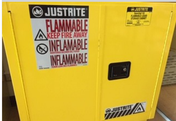
Example of a flammable cabinet.
