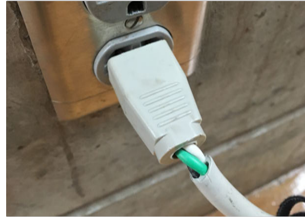
Always do a pre-use inspection of tools! Do not use and report if damaged!
