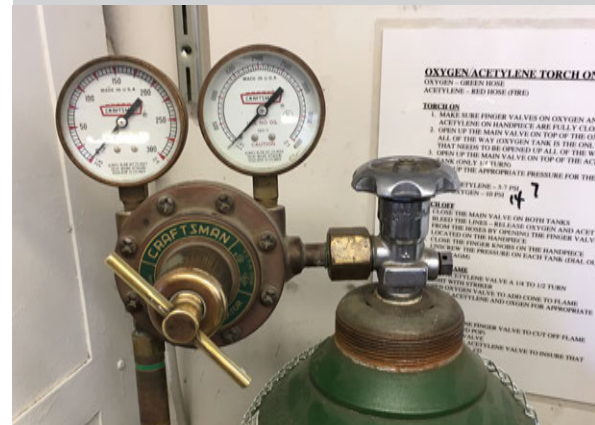
Turn valve off before attaching or detaching regulators!
