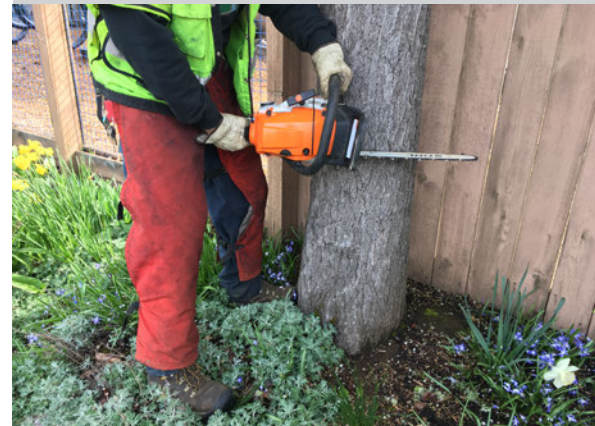
Keep a solid footing and use both hands to maintain control of the saw!
