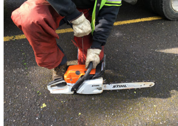
Always start two-handed on the ground with the chain brake engaged!
