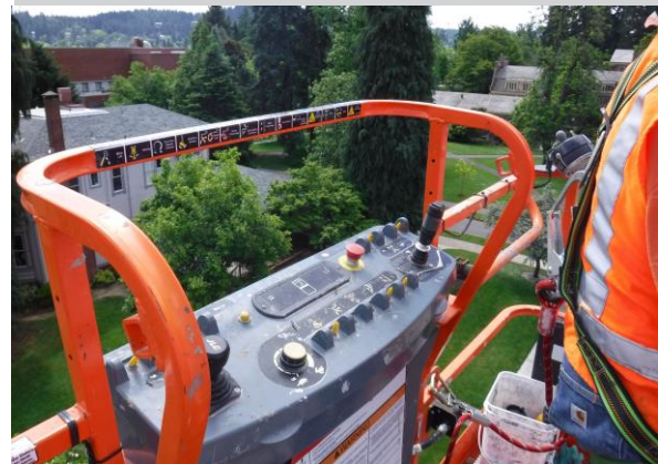
Wear required fall protection and a hard hat!
