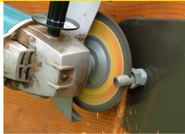
Ring test new or potentially damaged wheels!
