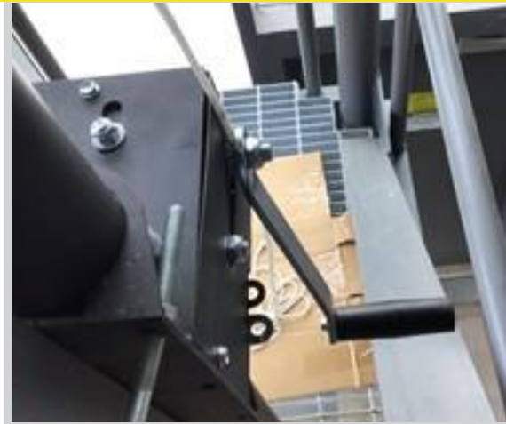
The tabs are not in alignment, so the crank can be turned.
